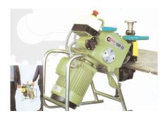
PR012-C – Power FeedBevel at 10 feet per minute
